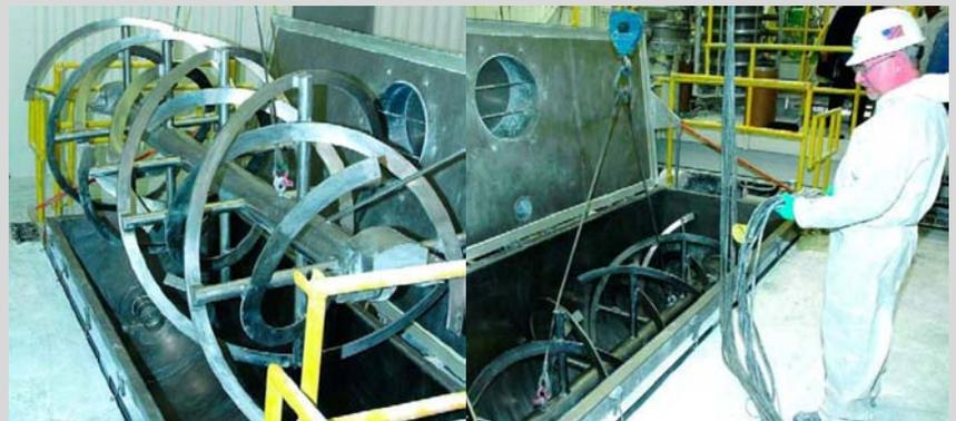
**Ross Ribbon Blender with removable ribbon agitator.** The ribbon is hoisted out of the blender using an overhead crane so operators can quickly and easily clean both the ribbon agitator and the trough.
